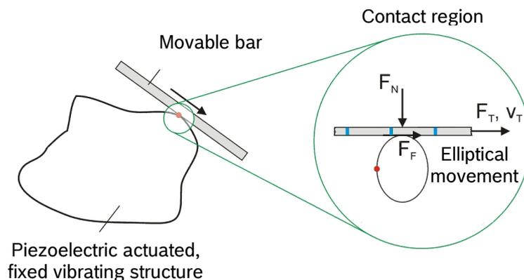
**Fig. 1:** Working principle of a piezoelectric micro-push motor
